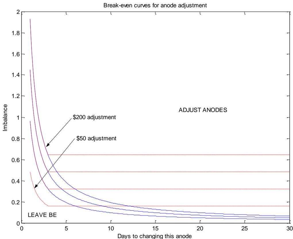
Figure 8. Break-even curves telling whether an anode should be adjusted in position or left alone. Blue solid line for persistent imbalance; red broken line for three day imbalance.
