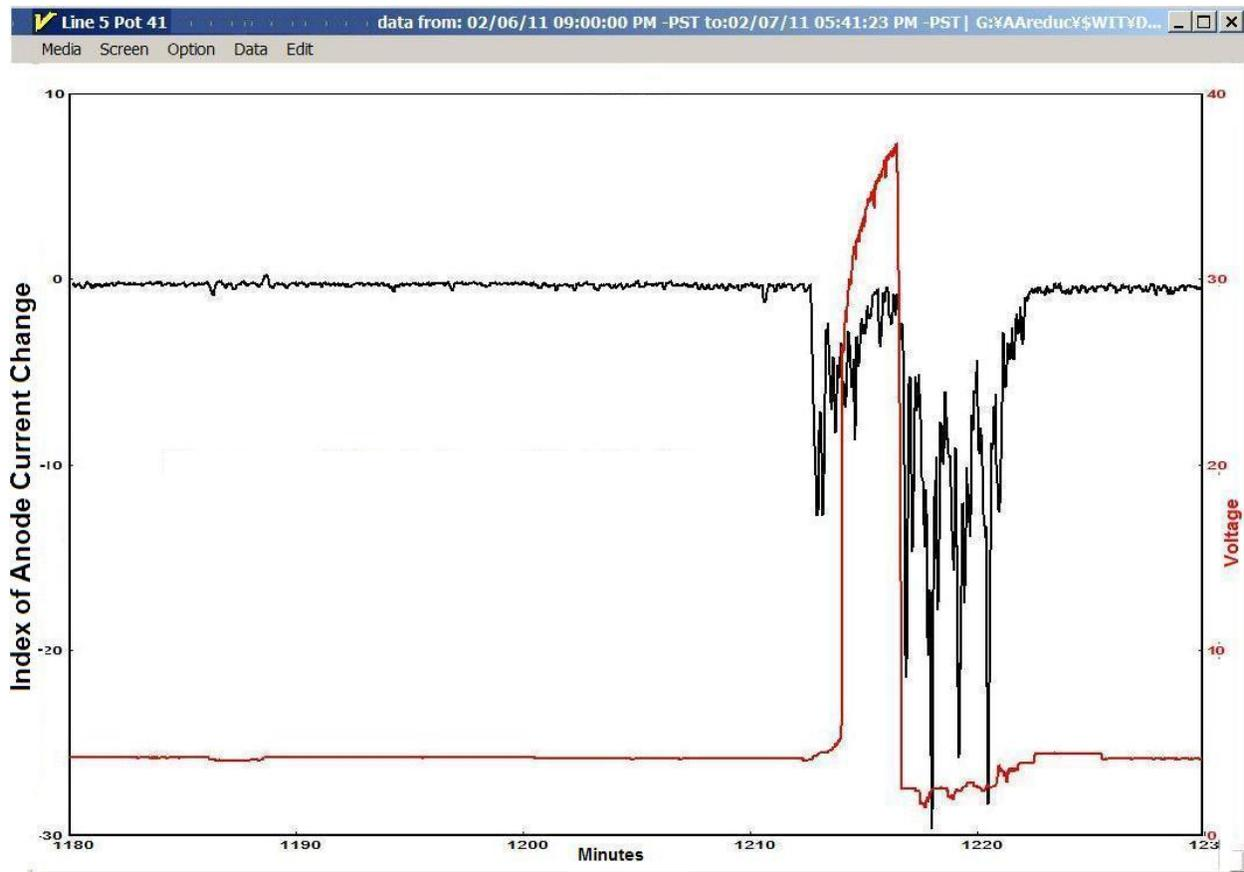
Figure 6. Representative plot showing early warning of anode effect from anode current distribution (blue line) compared to the pot voltage (red line)
