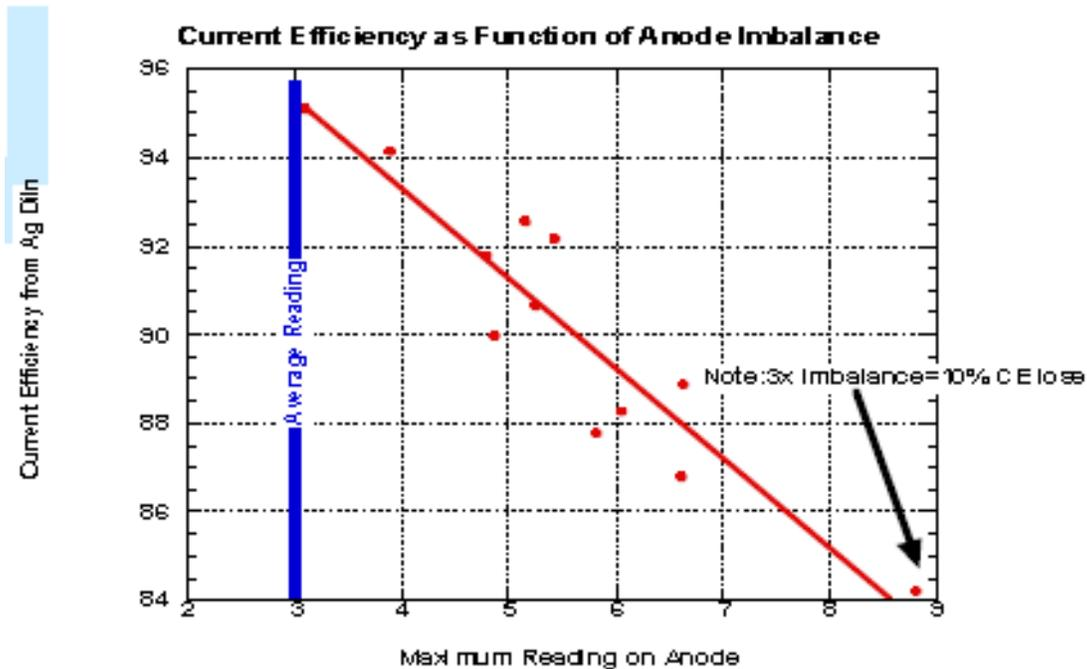
Figure 7. Measurements made by Tarcy on the effect of anode current skewness on CE
