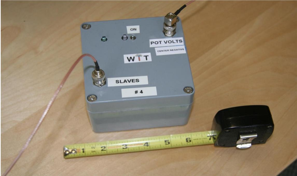
Figure 2. A “master” to be located at the end of the pot. Connections to the slaves and to pot voltage are shown. The master communicates wirelessly with a nearby computer.
