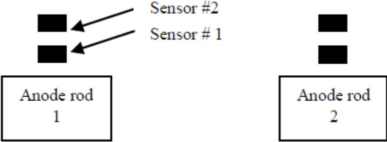
Figure 3. Schematic diagram of two anode rods, seen from above, each with two magnetic field sensors.
