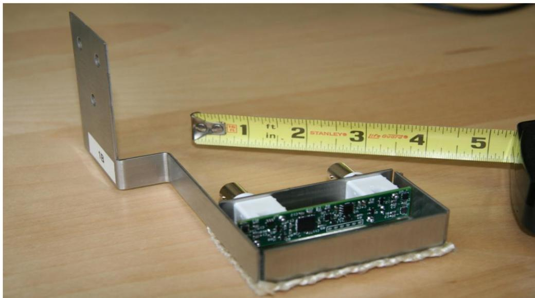
Figure 1. A “slave” used to measure the magnetic field produced by an anode current and thereby the current. The scale is in insulation. Assembly completed by adding an insulated lid and attaching cables to the BNC connectors.
