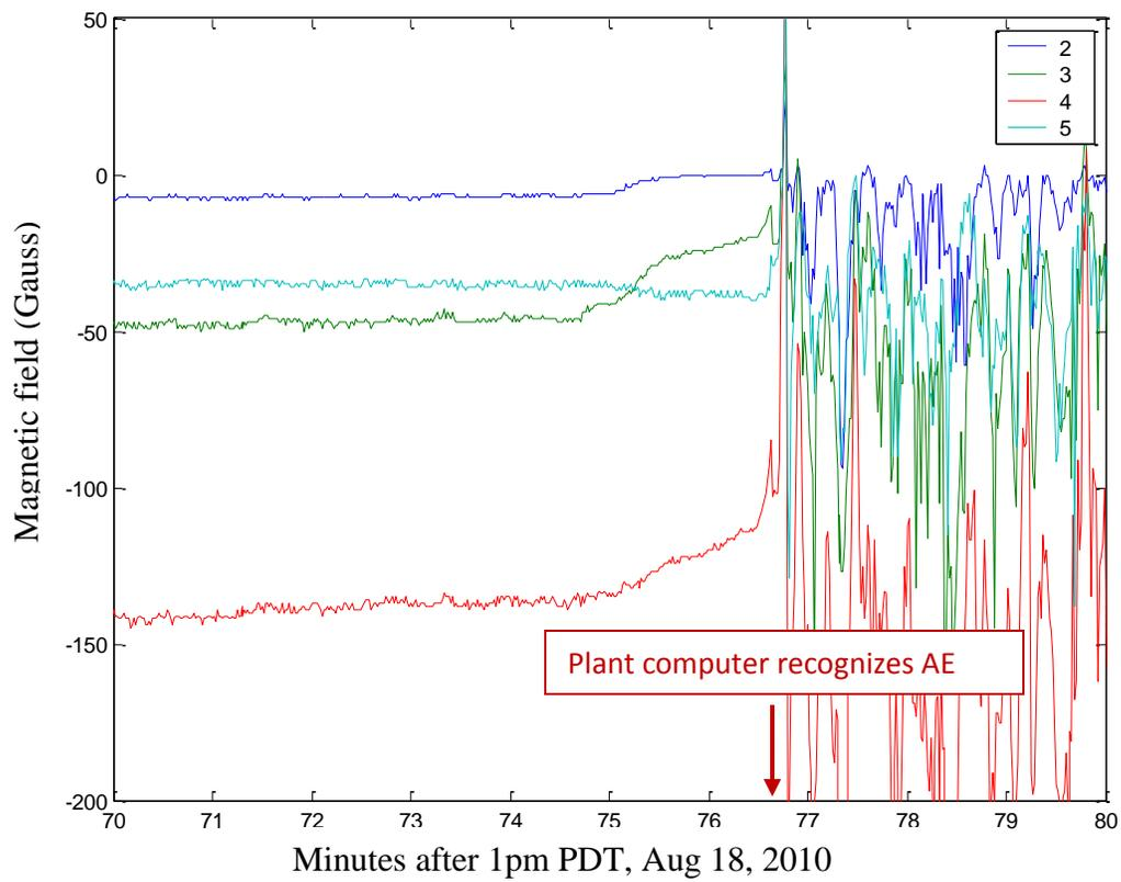
Figure 5. Traces of four anode currents (as reflected in magnetic field) as an anode effect starts – data from August test.
