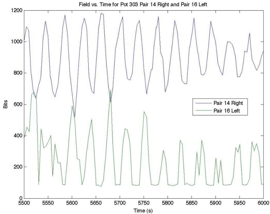
Figure 2. Magnetic fields (reflecting anode current) at two well separated anodes during first test of prototype for current measurement device at plant A.
