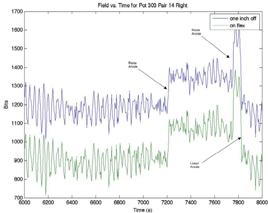
Figure 3. Current (magnetic field with “bits” diminishing as field increases) in an anode rod as the anode is raised or lowered.
