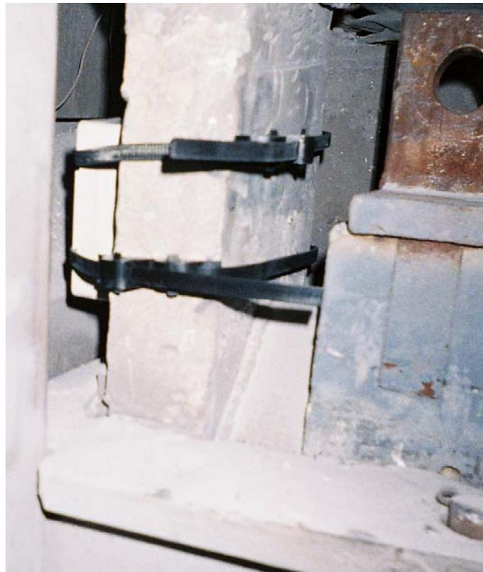
Figure 1. WIT mote attached to the tab at the end of an anode flex in plant A.
