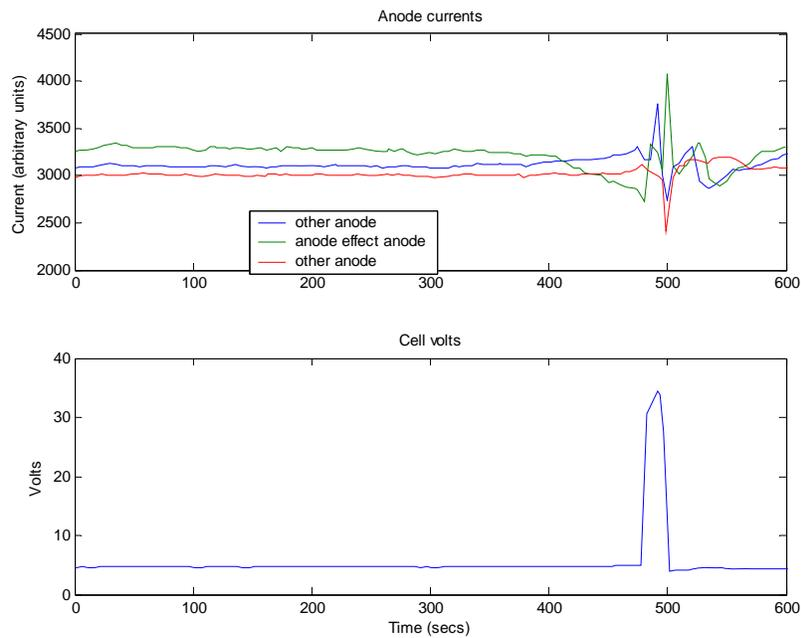
Figure 5. Cell voltage and anode currents measured wirelessly during a period when a cell underwent an anode effect.
