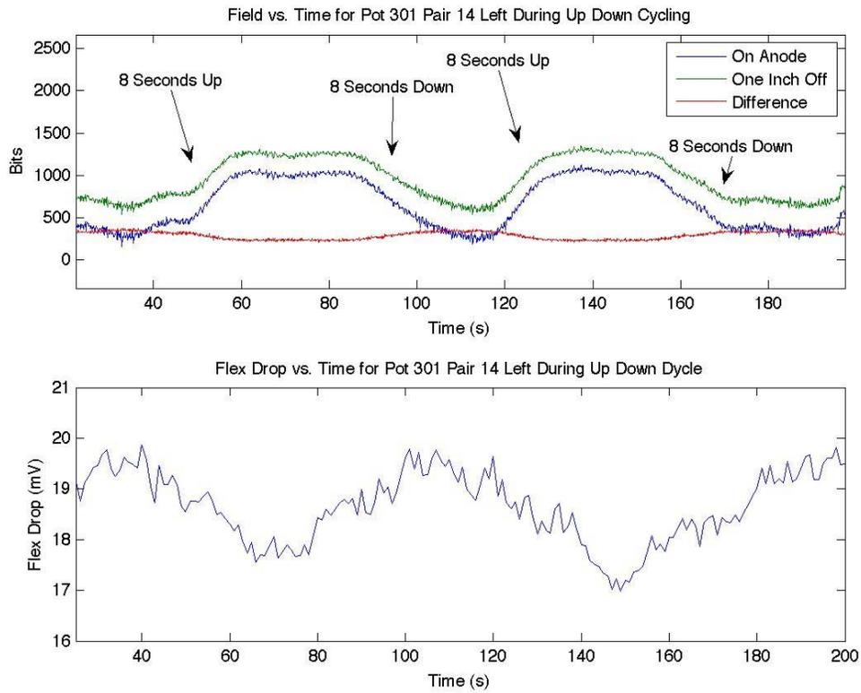
Figure 4. Comparison of anode current changes ascertained from WIT's mote measurement of field (decreased "bits" = more current) and those reported by the plant A computer (increased mV = more current). "Up" and "Down" refer to anode movements lasting the indicated time.
