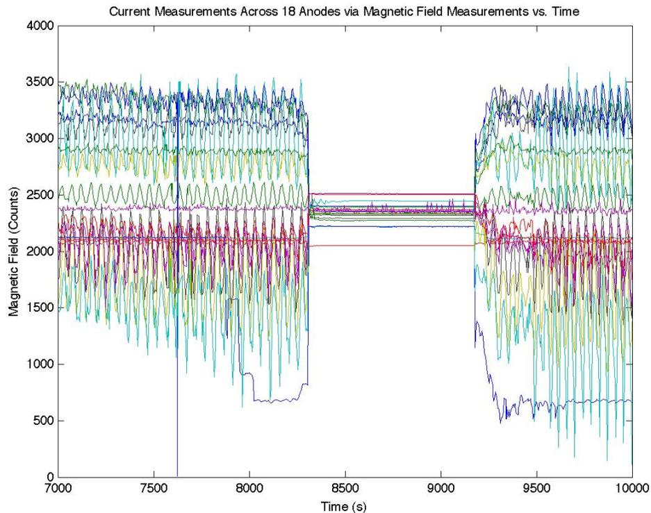
Figure 6. Currents (measured as magnetic fields) for 18 anodes on one pot measured during a 50 minute period where power to the pot was interrupted for about 15 minutes.
